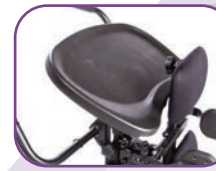
PA5716 Multi-Adjustable Black Molded Tray-11"Lx19"W Tray provides anterior support. Adjustable in depth, height and tray angle. Tray size is 11"Lx19"W (28x48cm).
