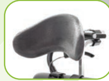
PY5626 Head Support 5"Hx8"W PY5628 Head Support 6"Hx10"W PY5630 Head Support 7"Hx14"W Cushion sizes are: PY5626 5"Hx8"W (13x20cm), PY5628 6"Hx10"W (15x25cm), PY5630 7"Hx14"W (18x36cm). Depth range is +1" to -2.75" (+2 to -7cm) from backrest. Maximum height from top of upper body pad is 10" (25cm).
