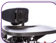
PA5751 Lateral Supports-4"-8" Range Curved Pads PA5752 Lateral Supports-7"-11" Range Curved Pad Keeps the upper torso in symmetrical alignment. PA5751 Adjustable from 4"-8" (10-20cm), PA5752 Adjustable from 7"-11" (18-28cm) with a 3.5" (9cm) height range. Pad size 4"Hx6"W (10x15cm).
