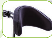
PA5586 Head Support-Form to Fit Cushion size 5"Hx10"W (13x25cm). Depth range is -2.5" (6cm) to +1.5" (4cm) from backrest. Maximum height from top of upper body pad is 10" (25cm).
