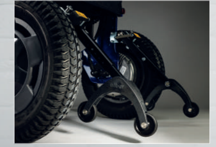
Premium anti-tipper option provides jack-up function for quick release of wheels
